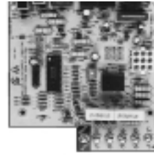
INTEGRATED FURNACE CONTROL
